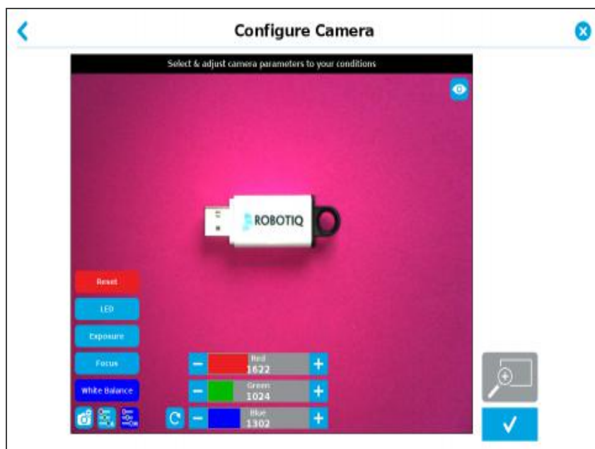
Fig. 4-24: Select Model step with White Balance option enabled (Manual mode enabled)
