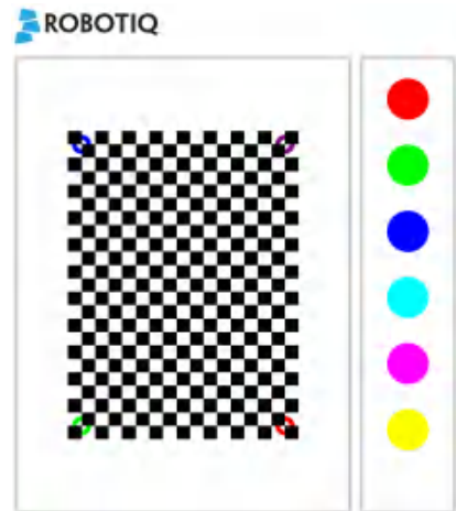
Fig. 4-8: Calibration board for UR3 Universal Robots models.
