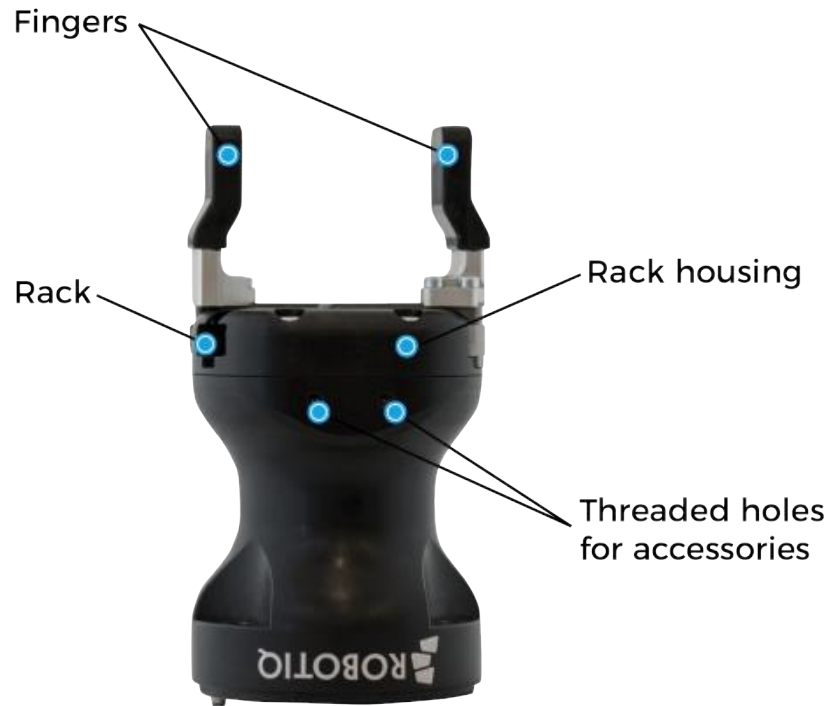
Fig. 1-1: Robotiq Hand-E Gripper.
